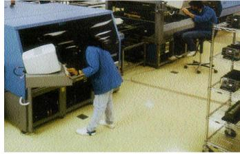
At Praegitzer's PCB manufacturing plant in Dallas, Oregon, Stonhard's Stonlux ATM flooring system effectively controls static and provides an attractive work setting.
